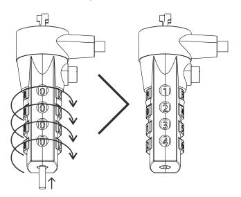
Use a small stick to push the button inside of the hole and hold it until you changed your combination. Release the button and new combination is set.
